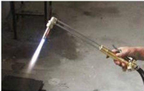
Exhibit 2 depicts an oxy-fuel cutting torch in action.
